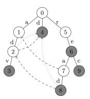
Figure 1: Illustration of trie and AC automaton of {"adv","d","re","read","rec"}: gray node denotes an ending of a pattern, dotted link represents *suffixP* pointer, and dashed link represents *fail* pointer. Pointers to the root are omitted.
