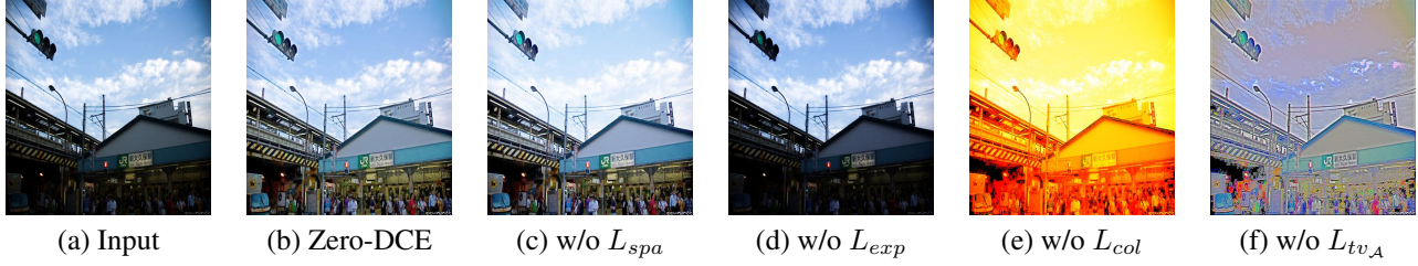
Figure 4: Ablation study of the contribution of each loss (spatial consistency loss L_{spa} , exposure control loss L_{exp} , color constancy loss L_{col} , illumination smoothness loss L_{tv_A} ).
