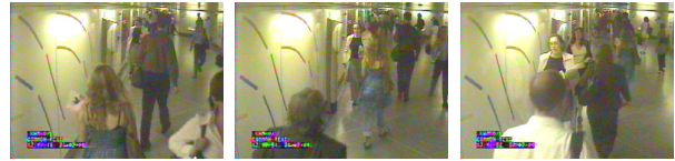
Figure 1. Three consecutive frames from a typical public space CCTV video where at a frame rate of 0.7 fps, an object can pass through the whole view in three frames.
