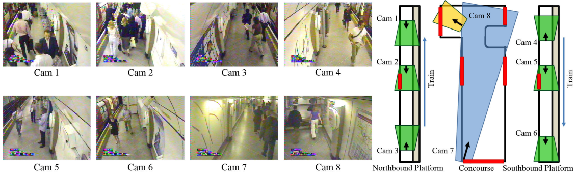
Figure 3. The layout of the underground station with the camera locations. Entry and exit points are highlighted in red colour.
